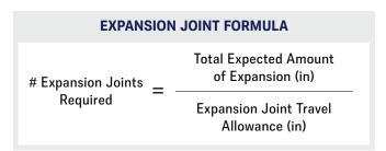
The number of expansion joints calculated above should be rounded up to the nearest whole number.
